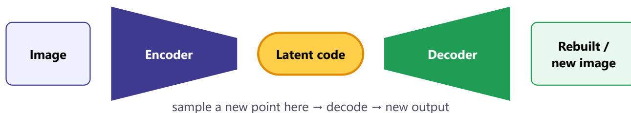
Figure 3.3 — A (variational) autoencoder compresses data to a latent code and decodes it back.
